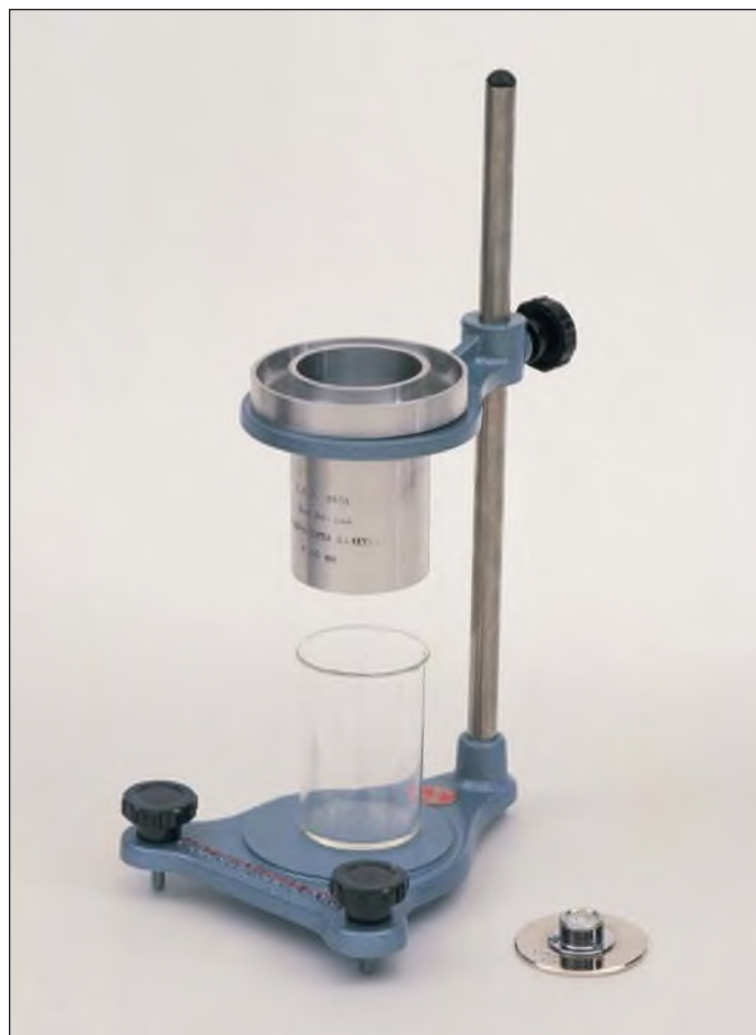
VC100 with stand, spirit level and beaker Flow cups VC120 and VC140 are similar
